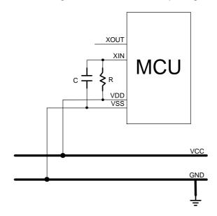
Note: Connect the R and C as near as possible to the VDD pin of micro-controller.
