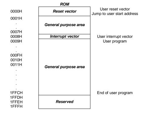
The ROM includes Reset vector, Interrupt vector, General purpose area and Reserved area. The Reset vector is program beginning address. The Interrupt vector is the head of interrupt service routine when any interrupt occurring. The General purpose area is main program area including main loop, sub-routines and data table.
