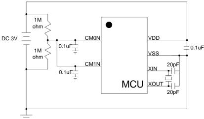
The application circuit use internal reference and the comparator output process by internal flag, so the circuit only uses CMnN pin to input battery 1/2 bias voltage to compare with internal reference voltage. Use comparator 0 to check battery 2.2V and comparator 1 to check battery 2.0V.
