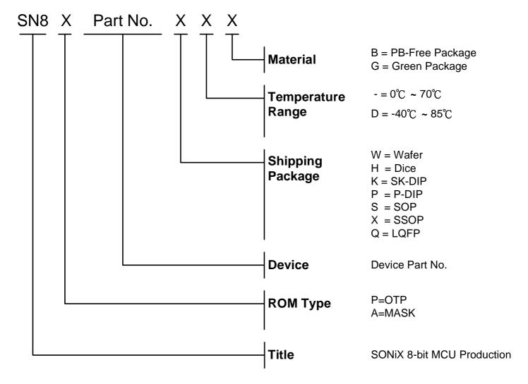
Note: SN8P26L34/26L32/26L321 doesn't support -40°C~85°C temperature range, LQFP package type and MASK ROM type.
