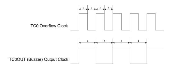
Example: Setup TC10UT output from TC1 to TC10UT (P5.3). The external high-speed clock is 4MHz. The TC10UT frequency is 0.5KHz. Because the TC10UT signal is divided by 2, set the TC1 clock to 1KHz. The TC1 clock source is from external oscillator clock. T0C rate is Fcpu/8. The TC1RATE2~TC1RATE1 = 101. TC1C = TC1R = 131.
