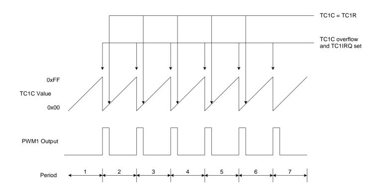
Above diagram is shown the waveform with fixed TC1R. In every TC1C overflow PWM output "High, when TC1C  $\geq$  TC1R PWM output "Low".
