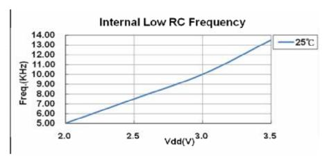
The internal low RC supports watchdog clock source and system slow mode controlled by CLKMD.
