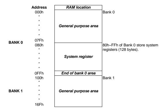
The 240-byte general purpose RAM is separated into Bank 0 and Bank 1. Accessing the two banks' RAM is controlled by "RBANK" register. When RBANK = 0, the program controls Bank 0 RAM directly. When RBANK = 1, the program controls Bank 1 RAM directly. Under one bank condition and need to access the other bank RAM, setup the RBANK register is necessary. Sonix provides "Bank 0" type instructions (e.g. b0mov, b0add, b0bts1, b0bset...) to control Bank 0 RAM in non-zero RAM bank condition directly.
